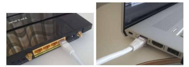
**IMPORTANT:** Make sure you connect the cable to a LAN port on the router (usually yellow), do not connect to a WAN port or Internet port (blue). Check the port labelling.
